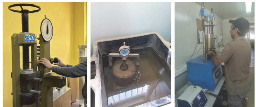
Figure 5. Laboratory examination of ITS (left) and CBR index with determination of linear swelling (center and right)
