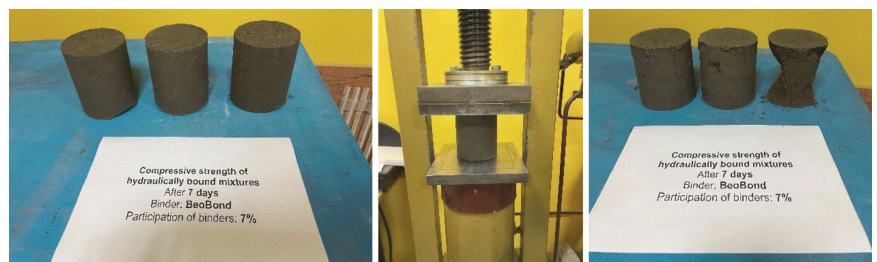
Figure 4. Samples stabilised with 7 % of BB binder before (left), during (middle) and after (right) UCS testing after 7 days of curing
